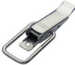
120mm Standard Toggle 308 grade stainless steel non locking version. Strength: 550kg
