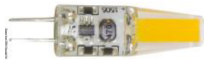
LED Light Bulb High-power SMD LED version. Screw G4. 12V. 1.6W. 18W Equivalent. 150 Lumens. 3000K 10 x 38mm Part No Description 70361 12V G4 Light Bulb 360° 1.6W
