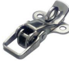
58mm Toggle + Eye 308 grade stainless steel locking version. Strength: 350kg
