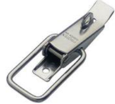
120mm Toggle + Eye 308 grade stainless steel locking version. Strength: 550kg
