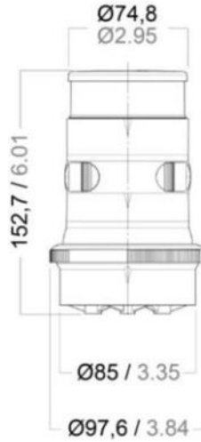
Tri Colour with Anchor Light Part No:70351
