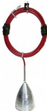
Zinc Hanging Anode. Kit includes 4 metres of cable with an M10 terminal, 1x mounting bracket and 2x re-useable rubber tie wraps. For use in Salt water.
